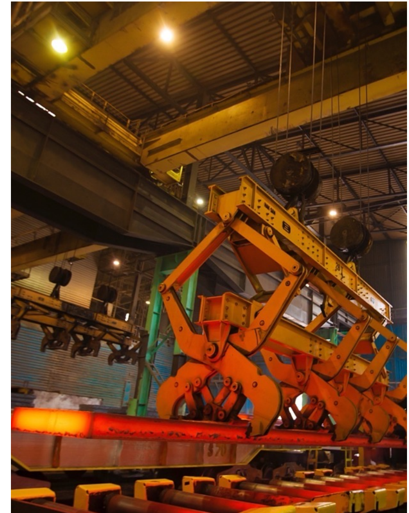
A crane lifts a hot steel slab to a cooling station at a steel plant in Germany
